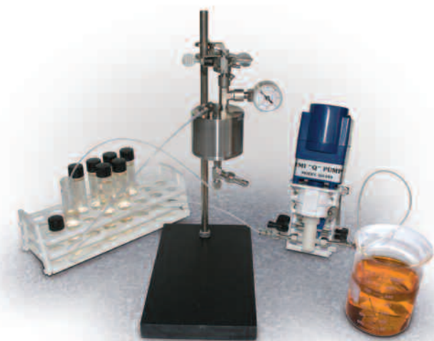
Lab cartridge test can be operated with pump (shown) or small pressure vessel.
